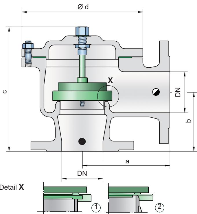
● = Tank connection for pressure relief function
