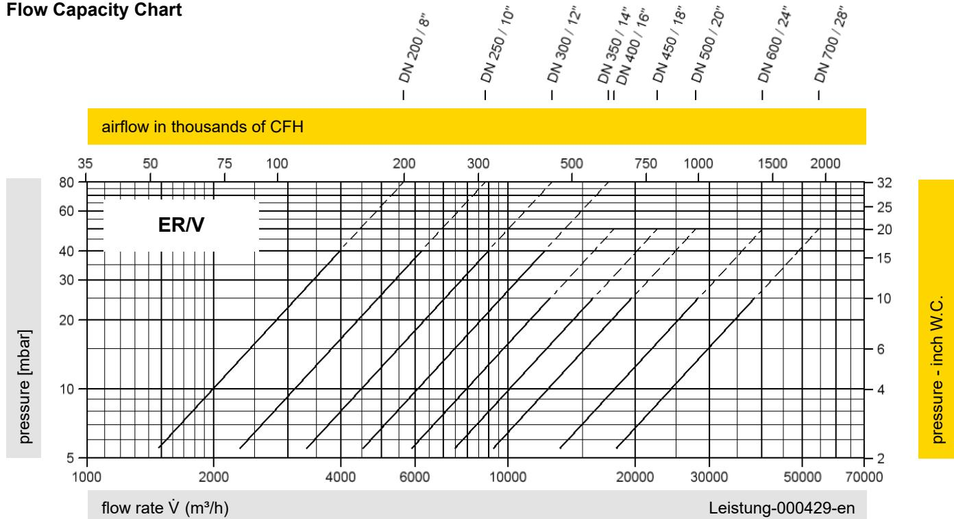
The flow capacity charts have been determined with a calibrated and TÜV certified flow capacity test rig.
